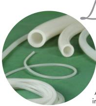
ow-volatile grade, platinum-cured silicone tubing is clean-room produced for critical pharmaceutical, biomedical, cosmetic, and food applications. APST has undergone extensive physical, chemical, and biological testing and meets USP Class VI, FDA CFR 177.2600, ISO 10993, European Pharmacopoeia 3.1.9, and 3-A standards.
